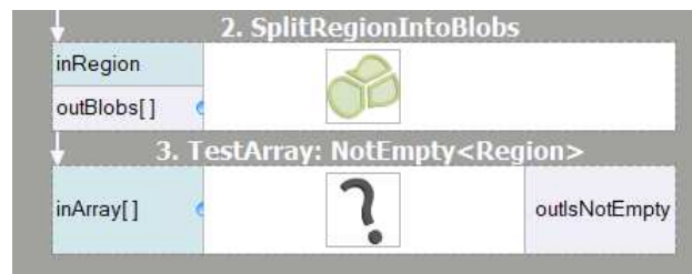
The TestArrayNotEmpty filter used to verify if there is at least one blob.
