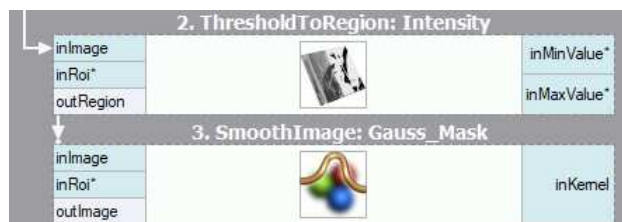
A typical example of automatic conversion: a region being used as an image.
